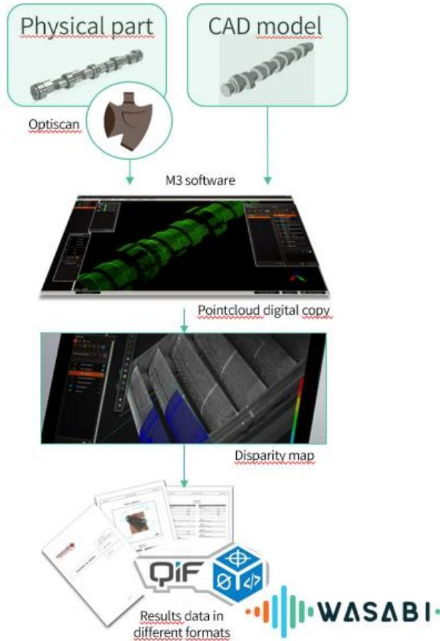
Figure 22: AS-IS Measurement process with CAD and M3 software
